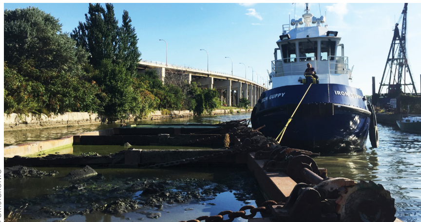
PortsToronto's Iron Guppy departing from the Keating channel with a loaded dump scow full of dredged material.
