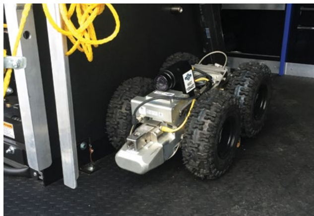
Small remote-control vehicles have been purchased by the port to go through all the stormwater lines.
