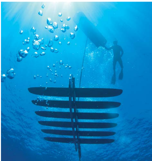
The robotic Wave Glider uses wave and solar power to travel long distances.
