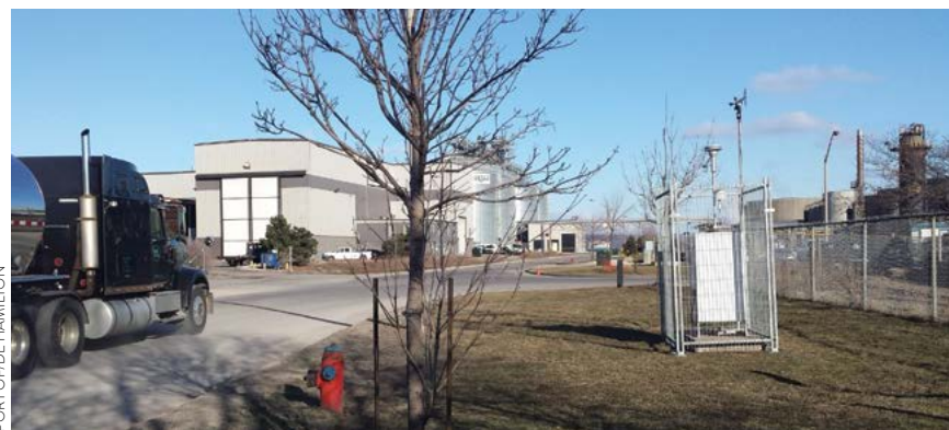
This air quality station monitors particulate matter (a Level 3 Green Marine criterion) at Eastport Blvd. in Hamilton, Ont.
