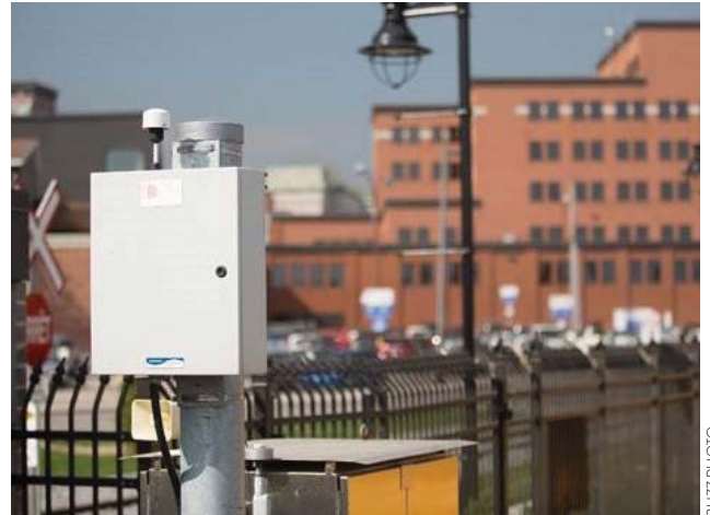
Dust detectors have been installed at the Port of Trois-Rivières to ensure good air quality and its monitoring in real time for the surrounding communities.
