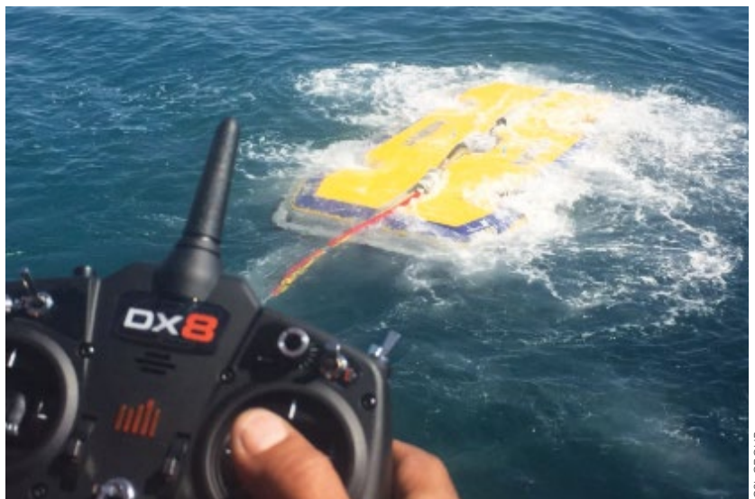
CSL Australia recently tried out a robotic hull cleaning system that automatically captures any loosened biofouling.
